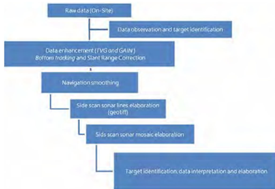
Figure 6 The general workflow for SSS data elaboration.
