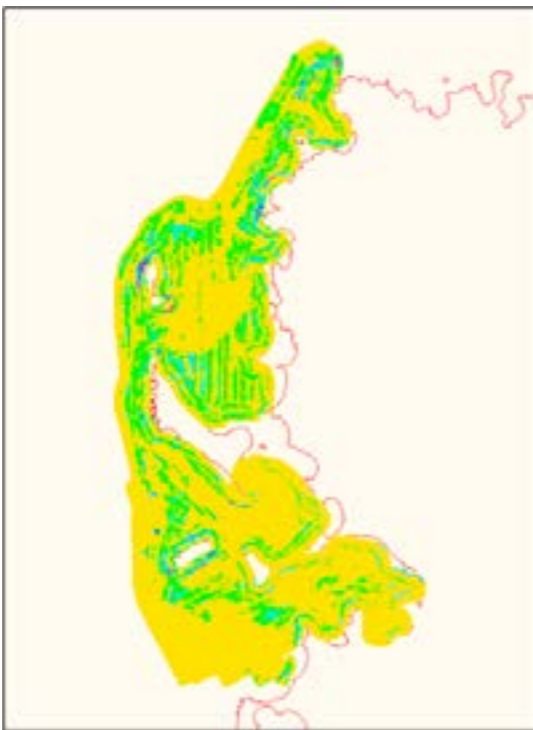
Figure 89 Trial two: Better result to determine the mud and hard bottom but bad at sandy and mixed sediment borders
