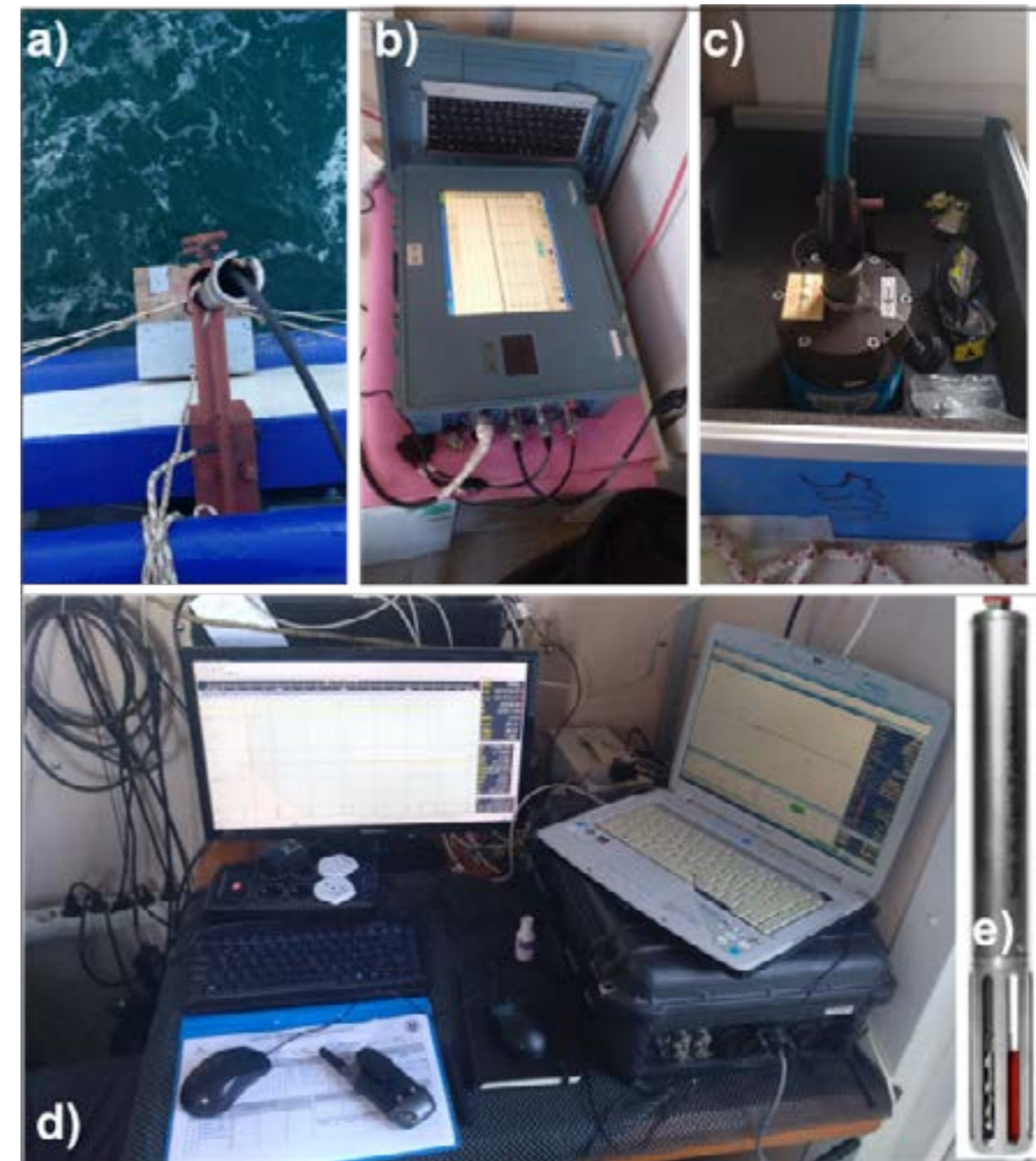
Figure 2 Data collection components a) Single Beam Echo Sounder Transducer, b) SBES System Unit, c) TSS motion sensor, d) NAVIPAC navigation system (left), Hydro Pro Data Collection System, e) CTD Probe
