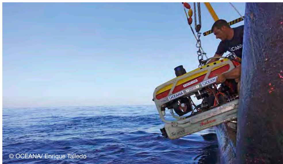
Figure 1. Remotely operated vehicle (ROV) on board the research vessel.
