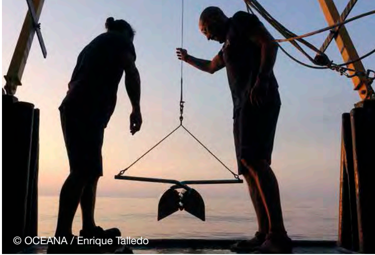
Figure 3. Preparation of the Van Veen grab for seabed sampling.
