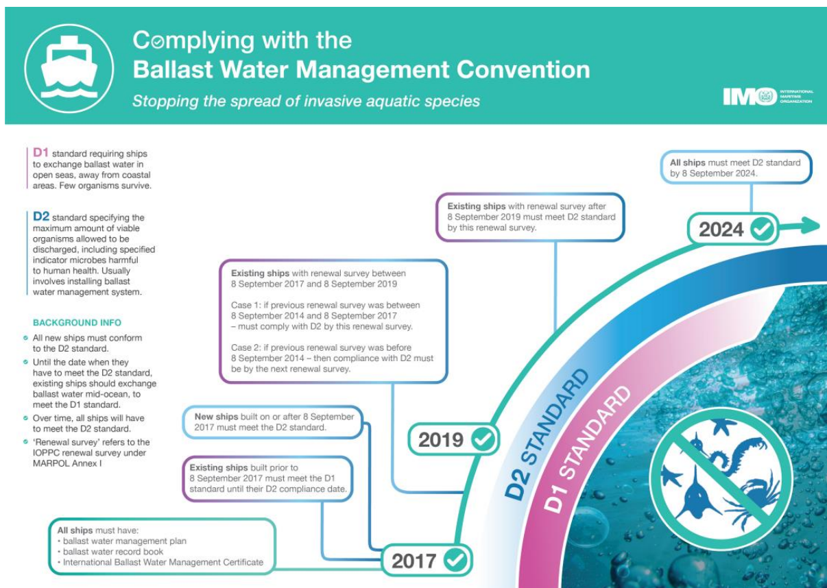
Figure 6: Infographic “Complying with the Ballast Water Management Convention”, from the IMO Website.
