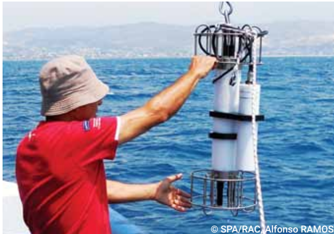
Figure 3.8. Launching the TCD off the stern of the oceanographic boat Cana .
