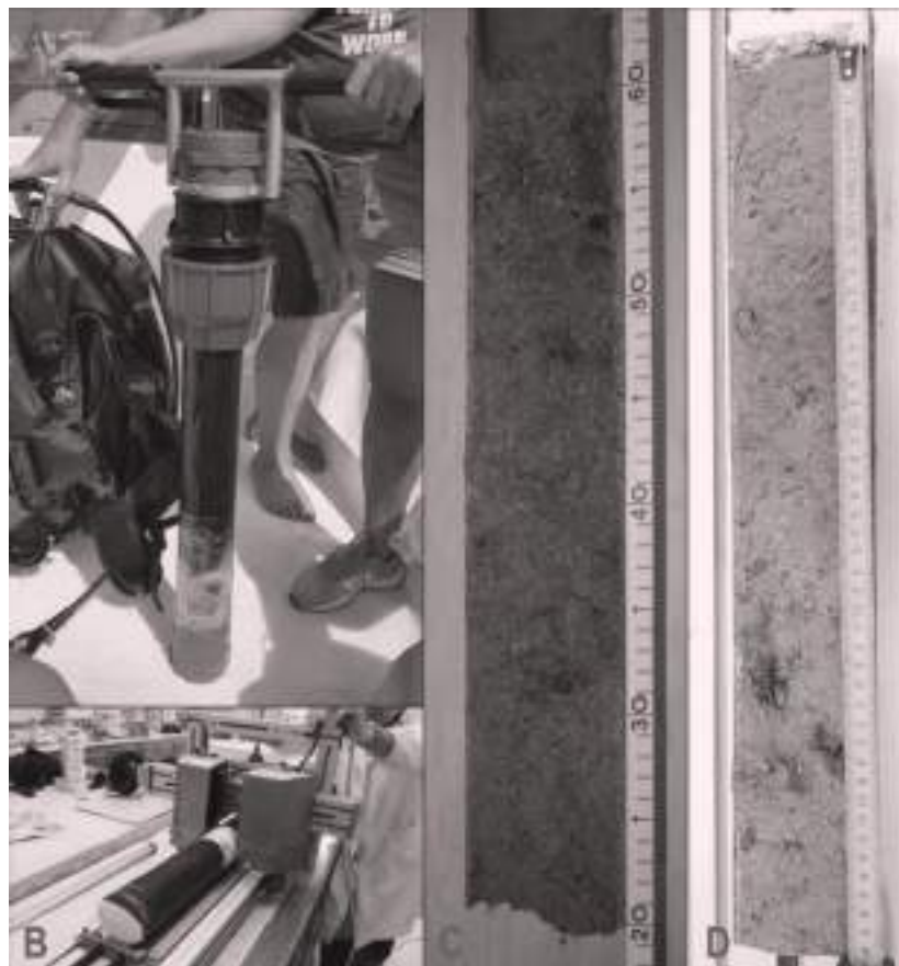
Fig. 1: A) Hand-corer used to collect the sediment cores; B) Instrument used for core sectioning; C) sectioned core (from 2018 sampling); D) sectioned core (from 2019 sampling).
