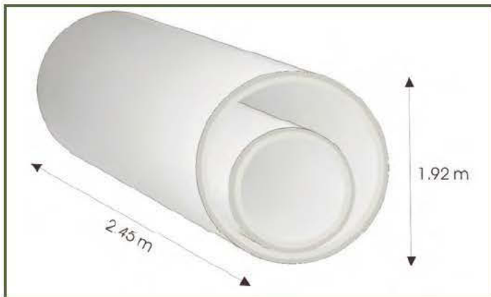
Fig. 91. Diagram of an artificial anti-trawl protection reef used in the Languedoc-Roussillon region (France). From Collart and Charbonnel (1998).
