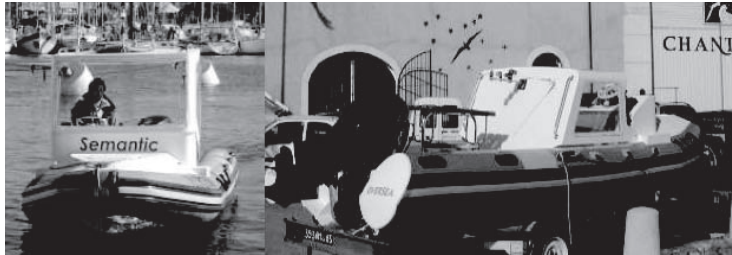
Fig. 1: Survey unit SEMANTIC : semi-rigid with removable cabin.
