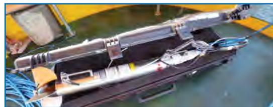
Acquiring acoustic images using a side scan sonar that enable types of habitat and geomorphologic features of the seabed to be made out
